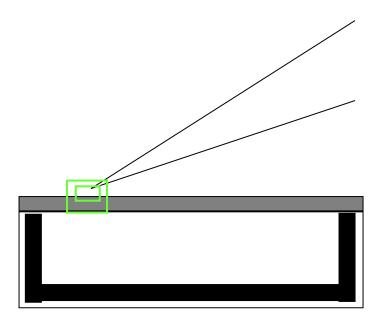
7. Cut the remaining "Pt bridges" free by serial milling with 100 – 500 pA and si.mtr. LOWER the stage until the sample is out of the trench. Put the Omniprobe in the parked location and retract the Omniprobe and the Pt GIS.
