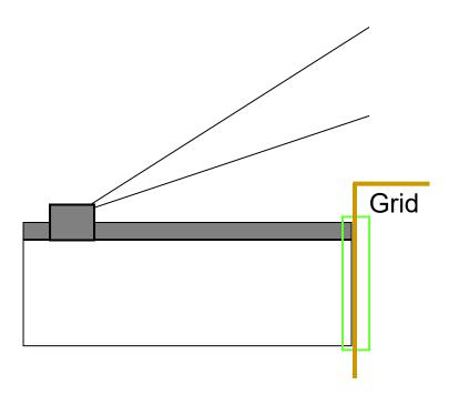
10. Tilt sample parallel to ion beam. Mill regular rectangles to cut lamellae thickness to < 1 um. Use aperture that gives a time between 2 and 8 minutes. For the front side, tilt the stage to 53.5°. On the backside, tilt the stage to 50.5° and rotate pattern 180°. These are the top and bottom of the lamellae when viewed in the i-beam.
